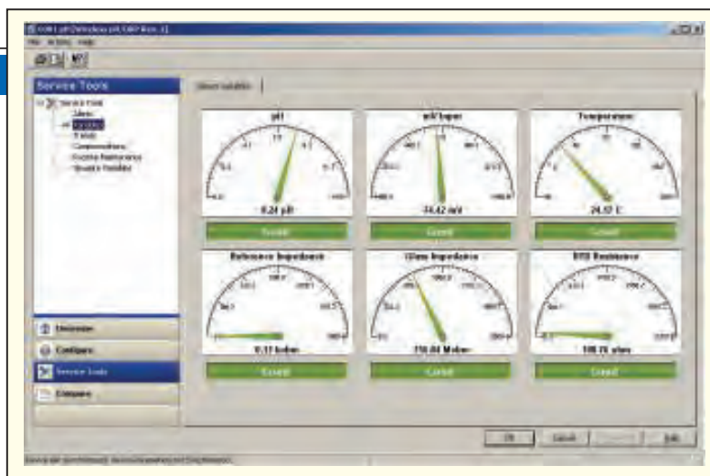
FIGURE 6. A software screenshot shows the health status of the pH-sensor in a process. These variables can be historized to see longer trends
