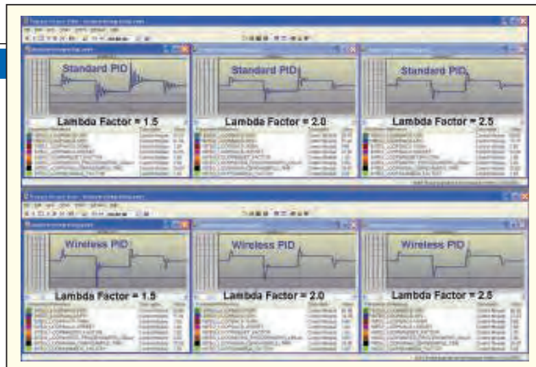
FIGURE 8. The enhanced, wireless PID performance (bottom row) has value beyond wireless operation by providing tighter and more stable control of processes with significant measurement delays from at-line analyzers. The Lambda factor is used for computing controller gain, and is inversely proportional to it
