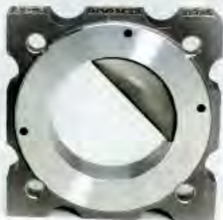
FIGURE 3. The partnership of CSI disk and CSR-7RS holder ensures that the disk bursts at or below its certified burst pressure even if the disk is installed in the wrong direction or becomes damaged
