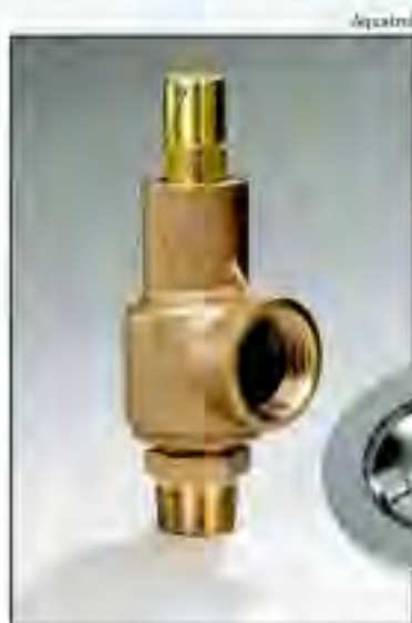
FIGURE 1. When a pressure relief valve pops, it recloses itself after having relieved the overpressure condition, enabling the system to continue operation
